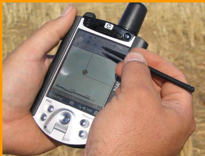
A GPS is used in the paddock to locate zones identified from yield maps and EM surveys
