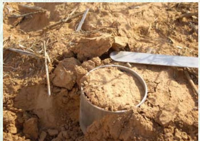
Soil core used to measure bulk density at the surface (0-5cm) after grazing, which had increased at both locations. Note the heavily crusted soil which had formed in the ungrazed area at Tootool. A slight crust had also formed at Greenethorpe, although this tended to disappear when wet.
