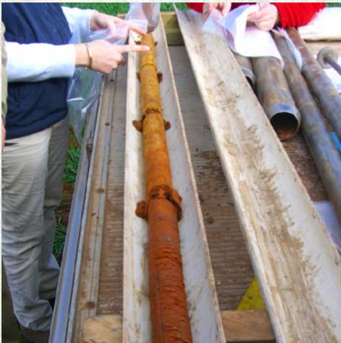
Soil core from Tootool - compaction in both paddocks was greatest at 10-20cm depth (penetrometer resistance > 3 MPa)
