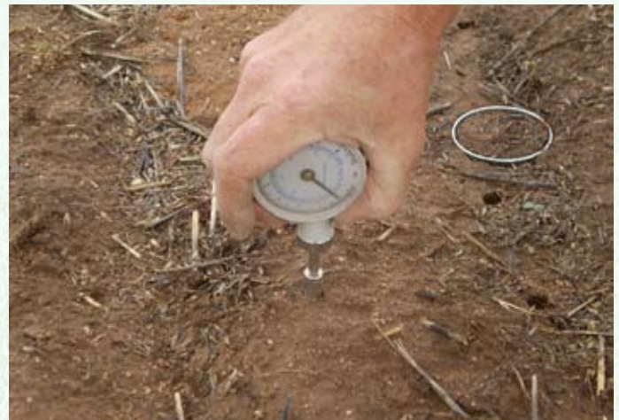
Penetrometer used to measure soil strength at the surface (0-1cm) after grazing, which had increased at Greenethorpe.
