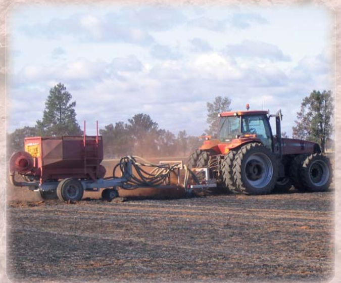
Yeomans deep ripper, modified with air hoses and cart for 'injecting' gypsum/lime to depth (FarmLink Zone Management project, 2005)
