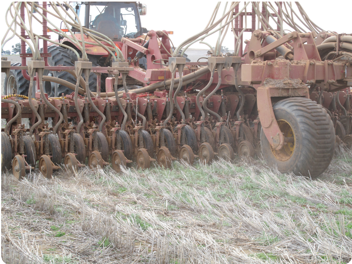
Disc seeding into stubble with low to moderate ryegrass numbers at the Grenfell trial, May 2010
