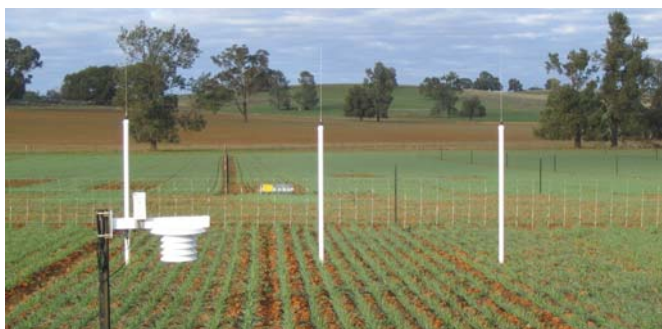
left: antennae used to radio data for each treatment from loggers to nearby receiver (Marrar)
