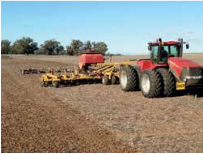
Figure 4. Dart's Serafin disc seeder and trailing rotary harrows (not photographed in trial paddock)
