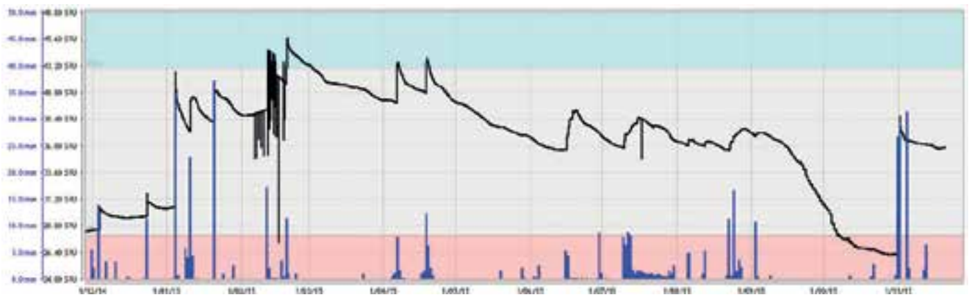
Figure 3. Denyer probe 1, Paw levels sum graph. Canola crop, January-December 2015. Blue bars = rainfall (mm).
