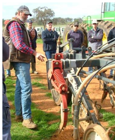
Photo 1 - Derek Ingold explains how he adapted sowing gear. Adapting equipment to give better trash flow was often the entry point into no-till farming Photo: Tony Pratt
