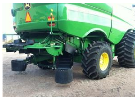
Narrow windrows for burning. Photo: Phil Bowden; and Chaff Deck fitted to JD header. Photo: AHRI.
