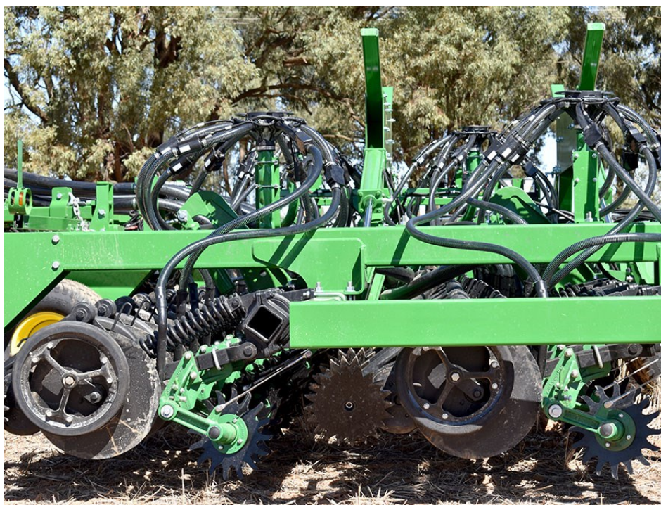
Photo 8 - Photo 18 Disc seeder with Aricks wheels to clear trash and prevent "hairpinning".
