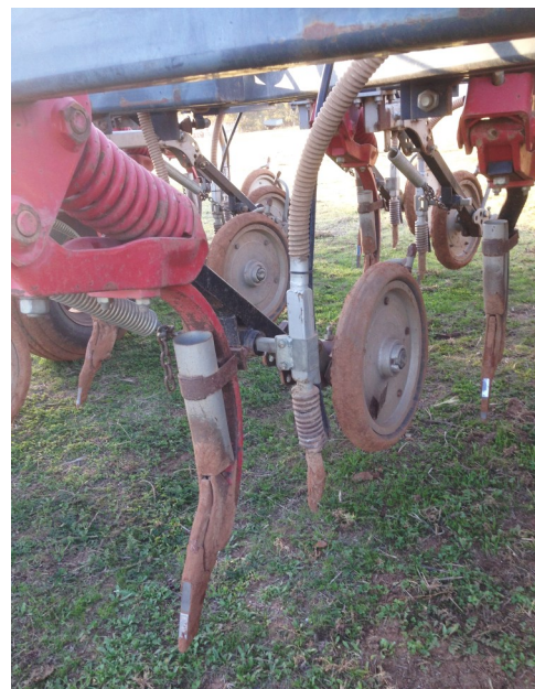
Photo 1 - Tine seeders have been modified to increase stubble handling capacity. Photo - Phil Bowden
