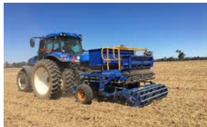
Figure 1. The 3-D Ripping Machine. The coulters in front of each ripping tyne and the back roller produce a flat seedbed. Photo by Guangdi Li
