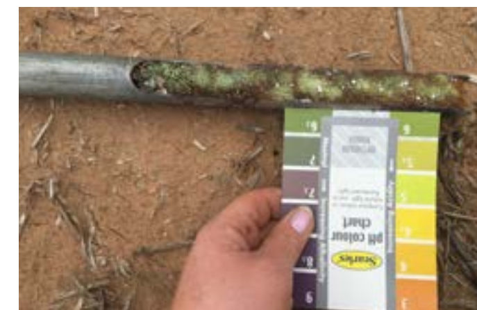
Image 1: Soil sampling and pH testing using a 'Dig stick' and off the shelf pH test kit.
