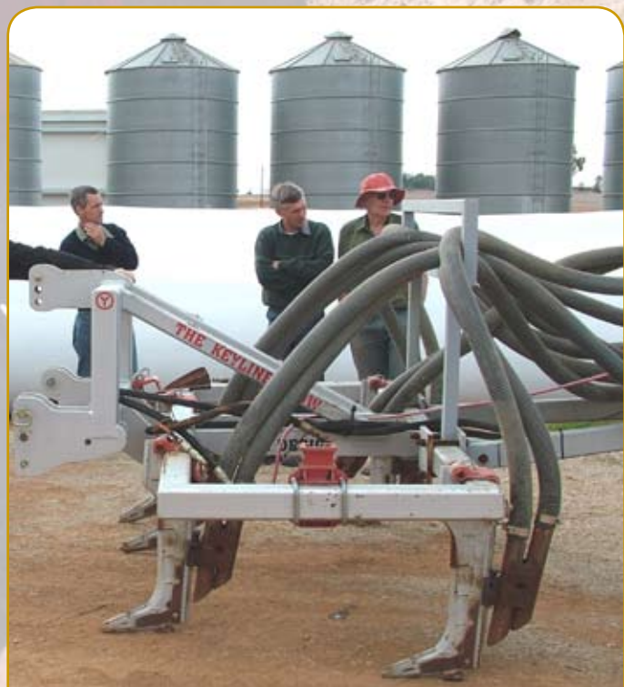
Figure 4. A deep ripper supplied by Yeomans Plow Co. was used to break up subsurface compaction at seven Canola in Depth trial sites. The tynes ripped to a depth of 30cm, at a row spacing of 45cm. Despite reducing compaction, no canola yield responses to deep ripping were recorded at any of the sites, suggesting canola is more tolerant of subsurface compaction than previously believed.
