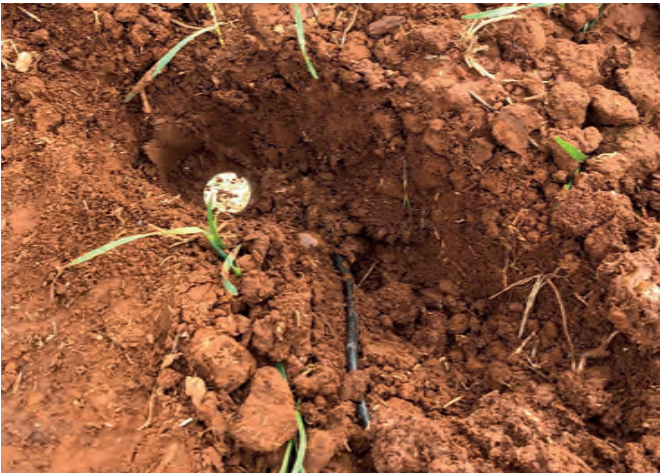
Figure 1. Installation of soil moisture probes at TAIC.
