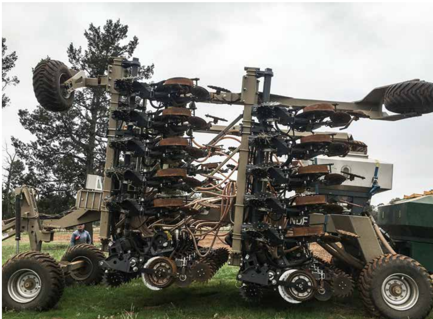
The NDF seeder featuring seed singulation technology which was used to plant a sowing strip trial at TAIC earlier this year. Adrian Roles will evaluate the trial at this year's FarmLink Open Day as a part of the CANOLA theme.
