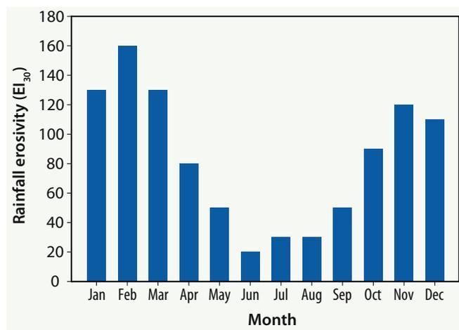
Figure 4 The approximate monthly erosivity of rainfall in the cropping areas of south western NSW. Erosivity is a measure of energy in rainfall and rainfall intensity. Actual erosion will depend on ground cover, slope and erodibility of the soil type (derived from Rosewell and Turner 1992).
