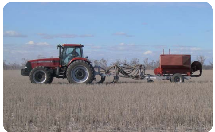
Fig. 1: FarmLink 'ripper/injector' used in the project. Modified Yeomans Plow rips to 30-40cm, placing gypsum/lime at 2 depth intervals above.
